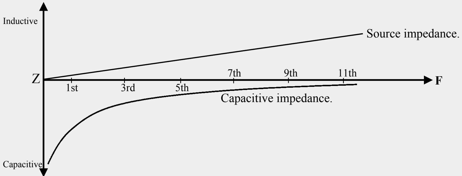
As the impedances offered at higher harmonics by the capacitor are far lesser than the other circuit impedances;
