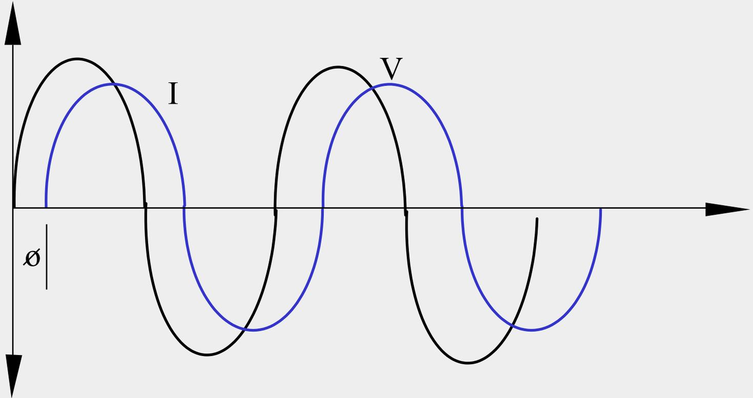
$$\text{Power Factor (P.F.)} = \cos \phi \quad (\text{as the waveforms are sinusoidal})$$
