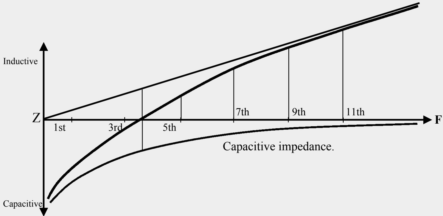
It can be therefore seen that impedance value offered by detuned capacitors is far higher than what is offered by plain capacitor.
