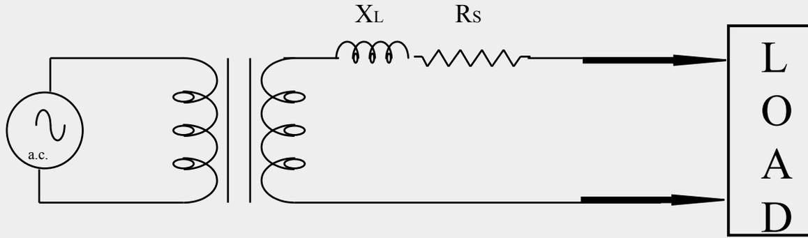
Here  $X_L$  is series inductive leakage reactance of the Transformer and  $R_s$  is the series resistance of the Transformer.
