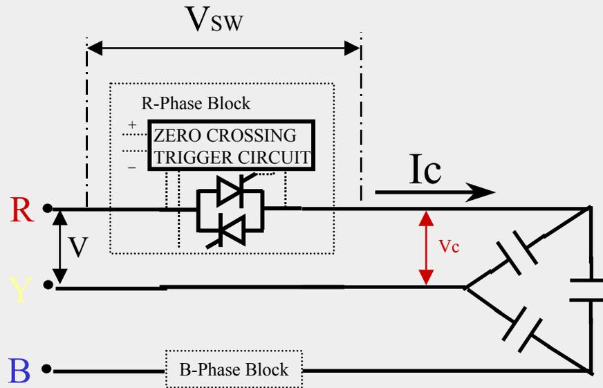
This clearly shows that the thyristorised switching along with the zero crossing detect circuit will bring the switching surge currents to almost nil.
