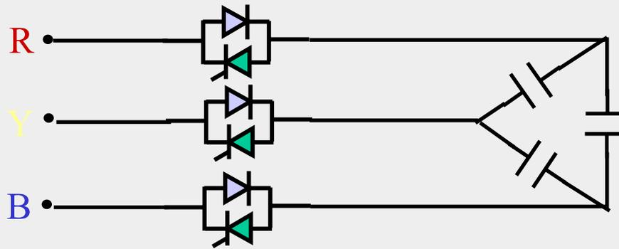
Back to back connected Thyristor and Diode blocks in all 3 Phases.
