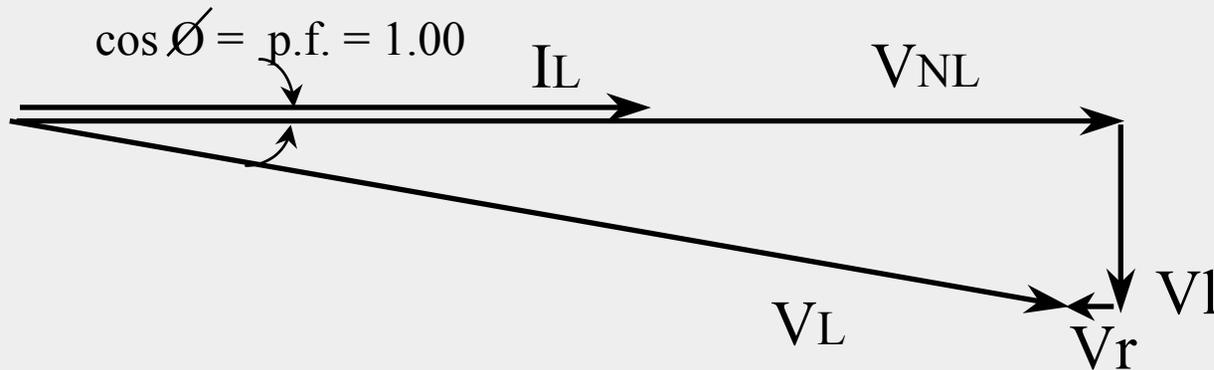
This clearly indicates the effect of poor p.f. on Voltage.
