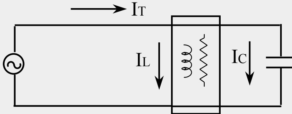
consider if the Capacitance inserted is lesser value, then  $I_C$  will be less , In that case p.f. will be lagging  $\neq 1$ .
