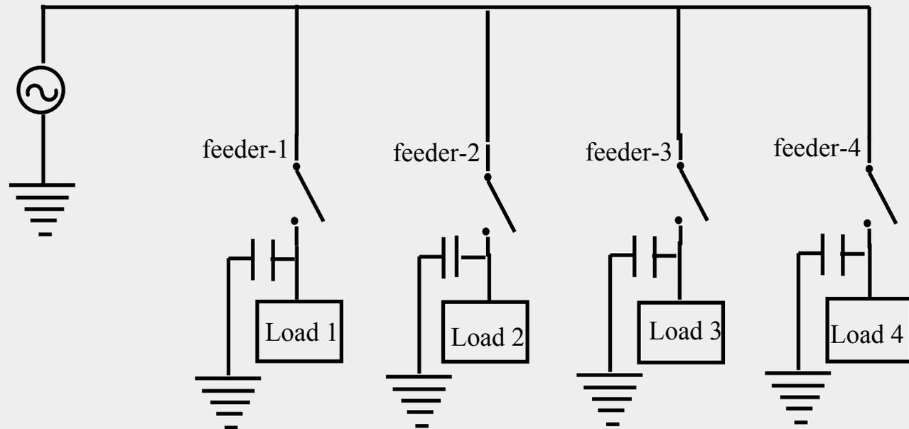
Here , every load is connected with just correct value of capacitor across it. So, when the load is put on, the capacitor also comes into the circuit.
