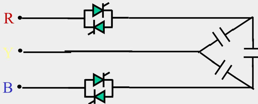
Back to back connected Thyristor blocks in only 2 out of the 3 Phases.
