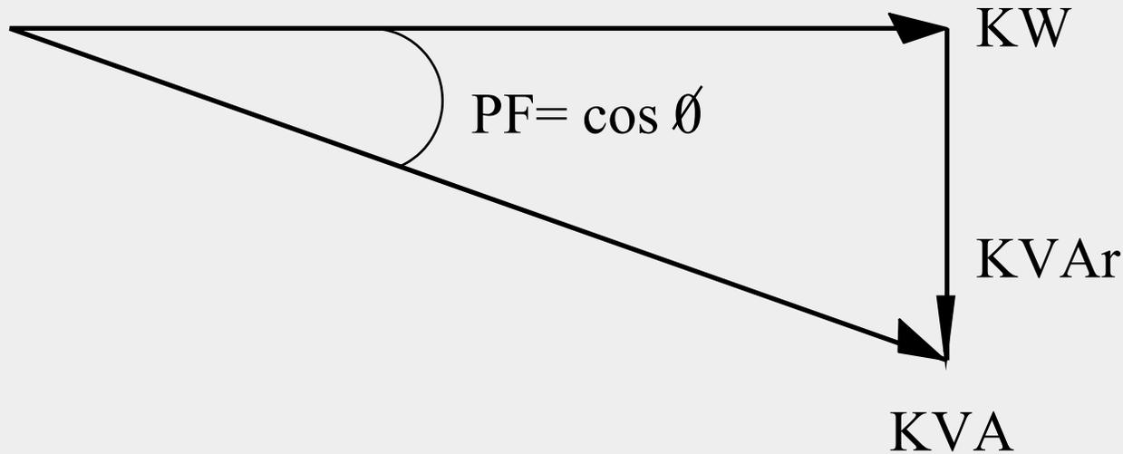
Power Factor is Real (Actual) Power divided by the Apparent Power. i.e.  $\text{KW}/\text{KVA} = \text{P.F.}$
